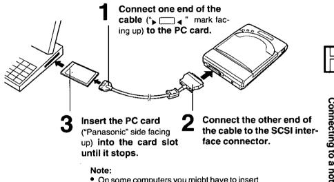
On some computers you might have to insert the PC card with the "Panasonic" side facing down. The card is keyed so it can only be installed in the correct direction.
